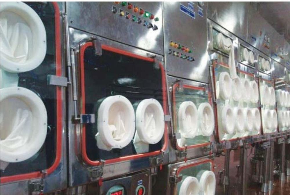
is preferable over glove ports as the operator extended reach/lift problem is largely eliminated.
